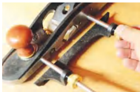
▲ Collet-style locking collars secure the fence to the bars at the desired position
